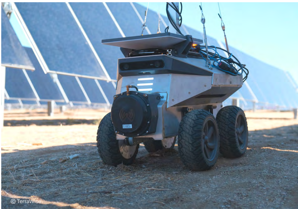
TerraWise's inspection robot autonomously performs quality checks during the construction process.
